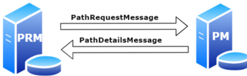
Figure 25 - Path Request Management module data exchange
